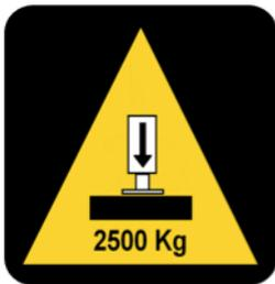
Use fixing points with sufficient stability. Consider every jack can lift up to 2500 kg. If necessary the fixing points at the chassis must reinforced with adequate parts.
