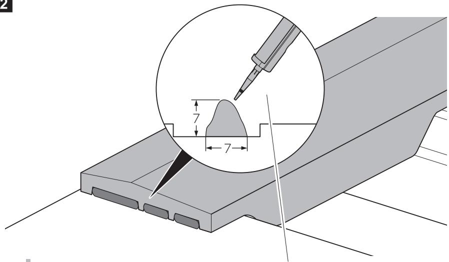
EN Recommendation: Malleable butyl sealant (e.g. SikaLastomer-710) or permanently elastic PU adhesive (e.g. Sika 221). Observe the preparation instructions given by the adhesive manufacturer.
