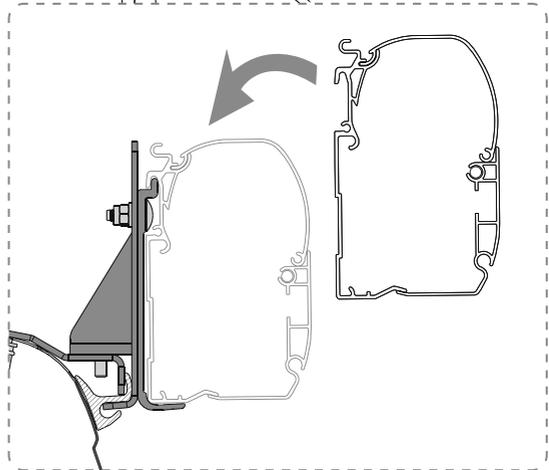
**EN** Before tightening the screws, make sure that the awning position doesn't prevent the opening of the rear door.
