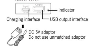
The green indicator flickers say power charging, green light going on say full with power. When the USB output interface is used for external equipment charging, the red indicator going the indicator flicker means power off.
