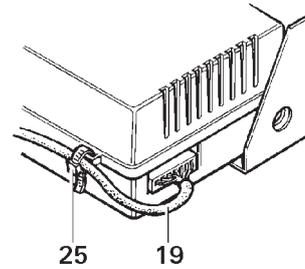
For strain relief, secure control panel cable (19) on the control electronics by means of enclosed cleat (25).
