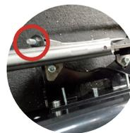
Setting screw for handbrake
