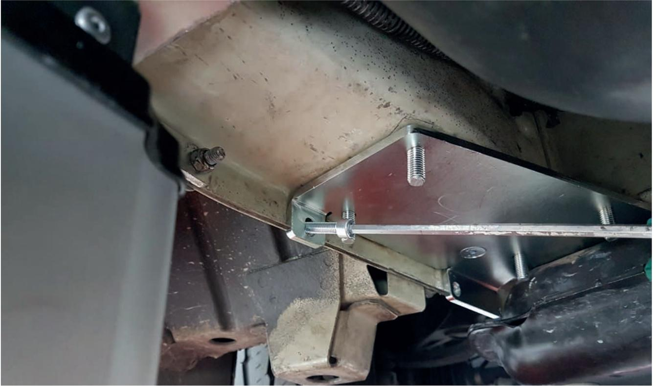
Fix the adapter plate with two M8 bolts on the chassis.
