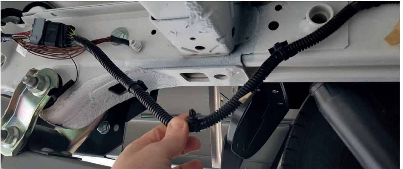
Move the electric wiring to the side, then insert the adapter.
