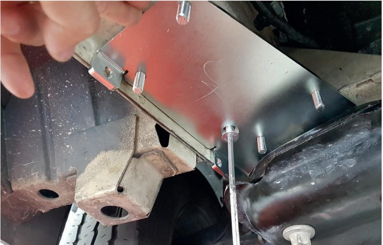
Fix the adapter with the mounting plate that you inserted into the hole.
